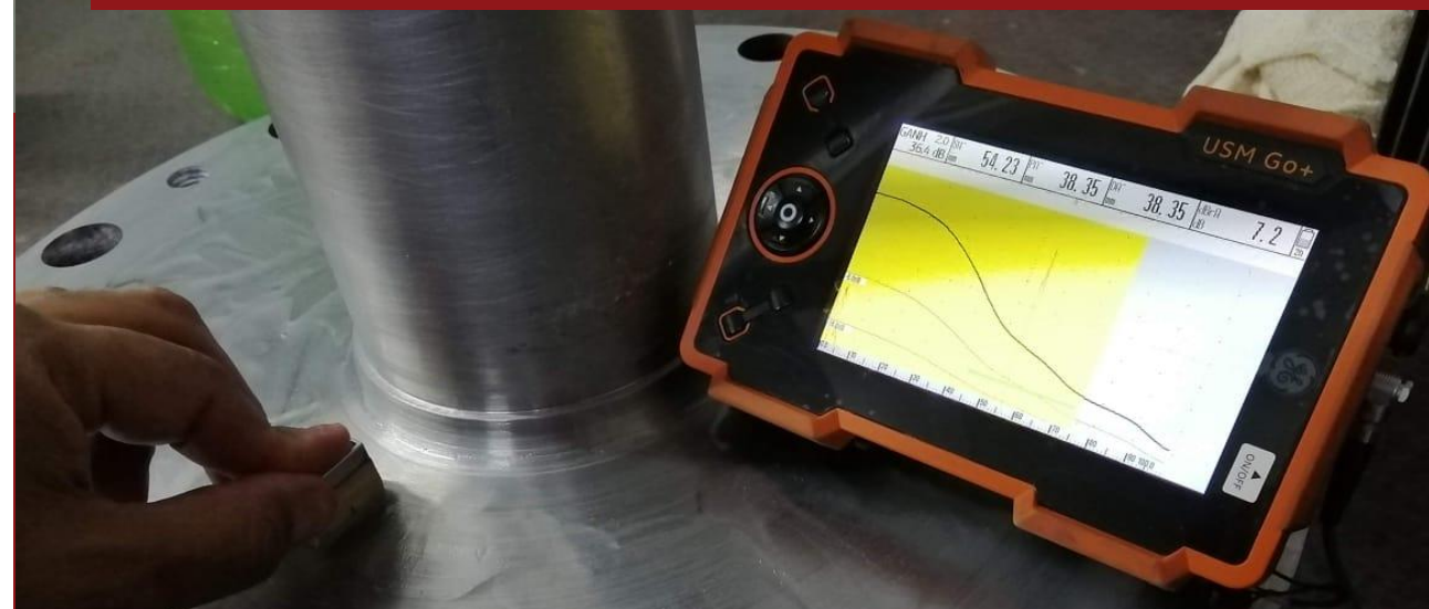
Ultrasonic inspection in clinker oven welding
