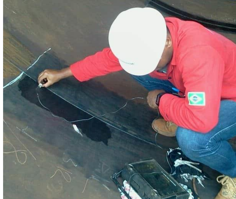
Ultrasonic inspection in clinker oven welding
